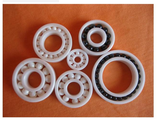
Full ceramic ball bearings constructed entirely of ceramic material. Inner/outer races and balls are made of Silicon Nitride (Si3N4) or Zirconium Oxide (ZrO2). They are available as full complement (no cage) or with a cage made from PEEK or PTFE. Full ceramic bearings are for medium load and medium speed applications. It is not possible to achieve the inner and outer ring roundness that is found with precision steel bearings, so full ceramic bearings have lower speed ratings.
